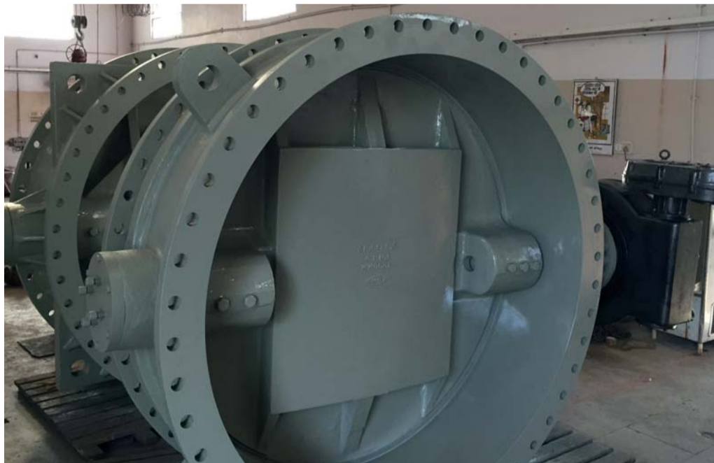
G M Engineering can make some very large valves indeed, and has delivered two-metre butterfly valves to a water projects in India
